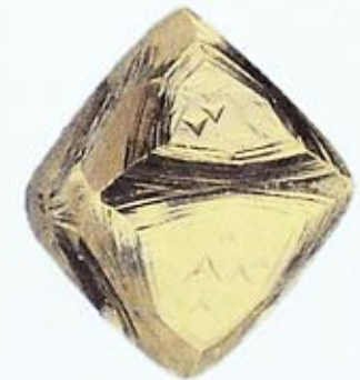
Crystal faces on a rough diamond with distinct trigons indicating its natural origin
